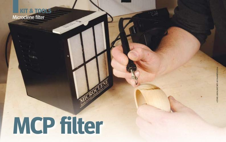
**Patricia Spero** looks at this specially dedicated pyrography filter from Microclene, manufactured by Acrol UK. The unit is quick and effective at removing smoke and fumes from the work area
